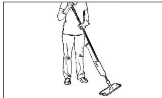
Figure 6. Applying floor finish with Flat Mop (optional)
